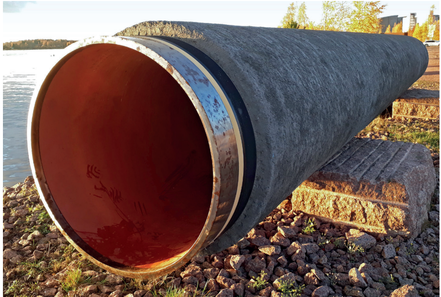
A section of steel pipe for Nord Stream 2 with concrete coating. (Photo: Wikipedia)
