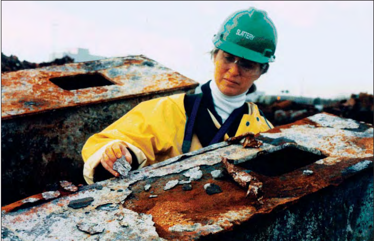
Figure D-16 Engineer inspecting fire damage of perimeter column tree from WTC 1 or WTC 2.
