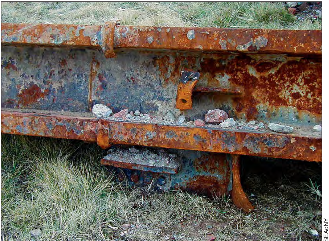
Figure D-17 Seat connection in fire-damaged W14 column from WTC 7.
