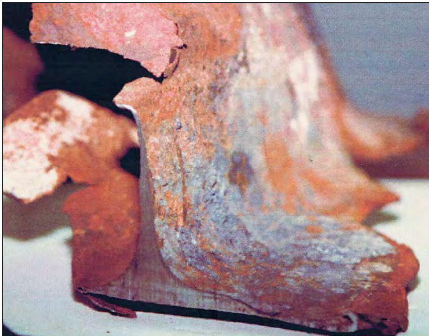
Figure C-2 Closeup view of eroded wide-flange beam section.
