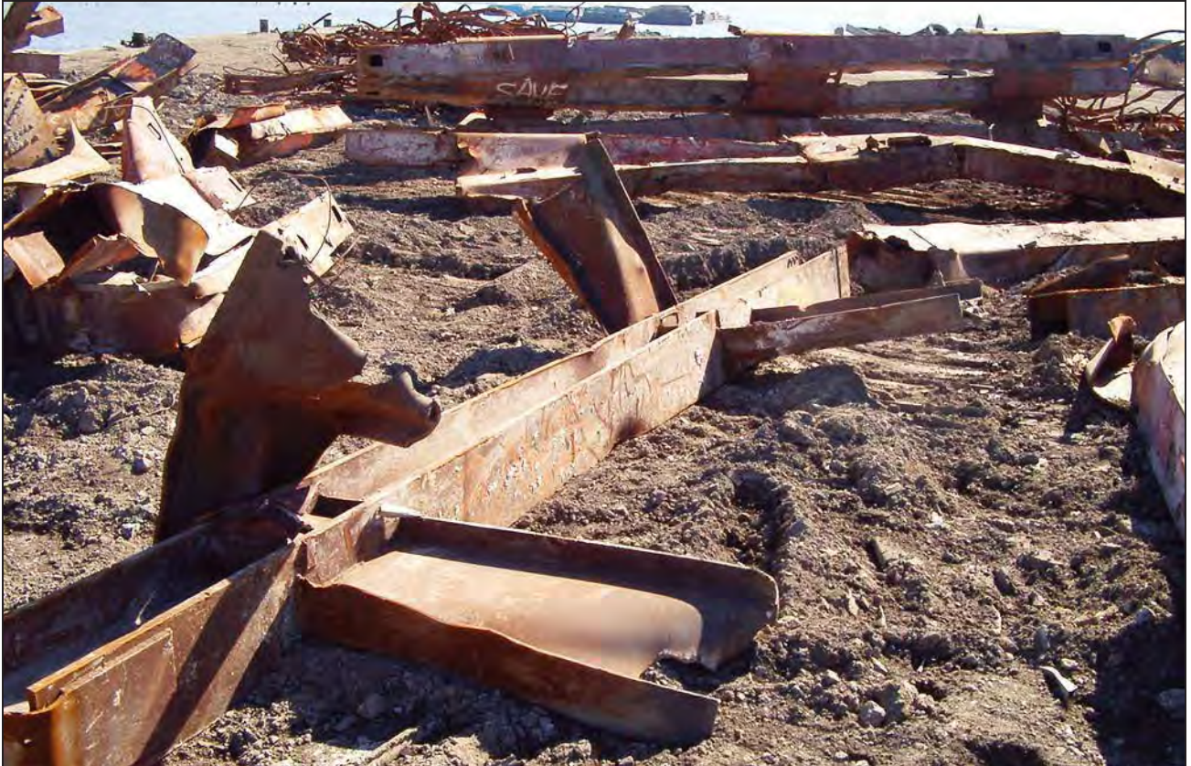
Figure D-14 WTC 7 W14 column tree with beams attached to two floors.
