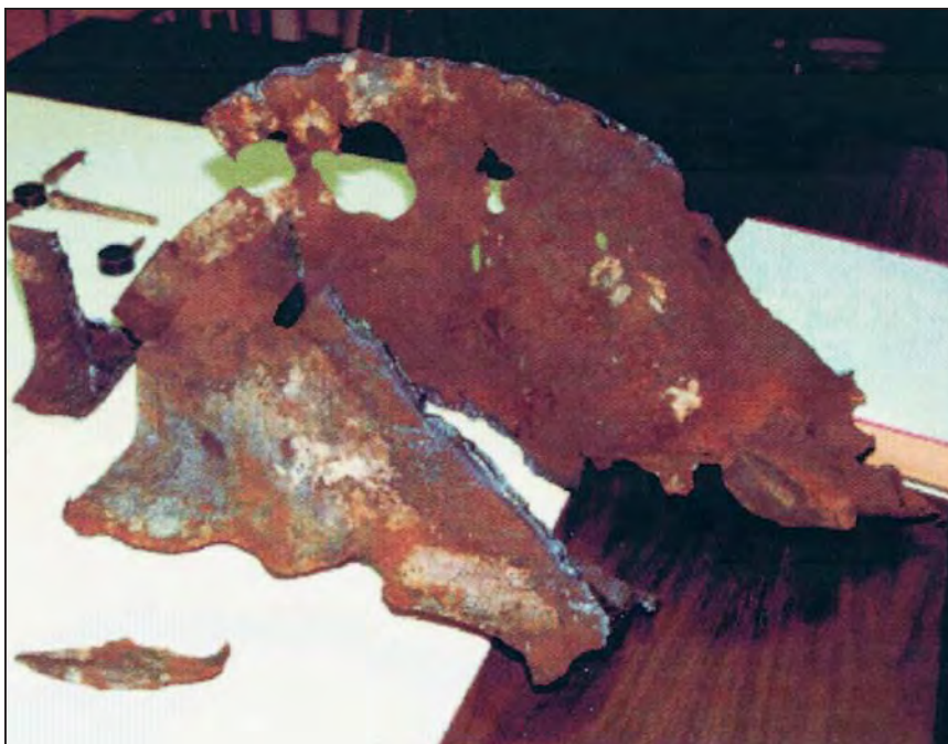
Figure C-1 Eroded A36 wide-flange beam.
