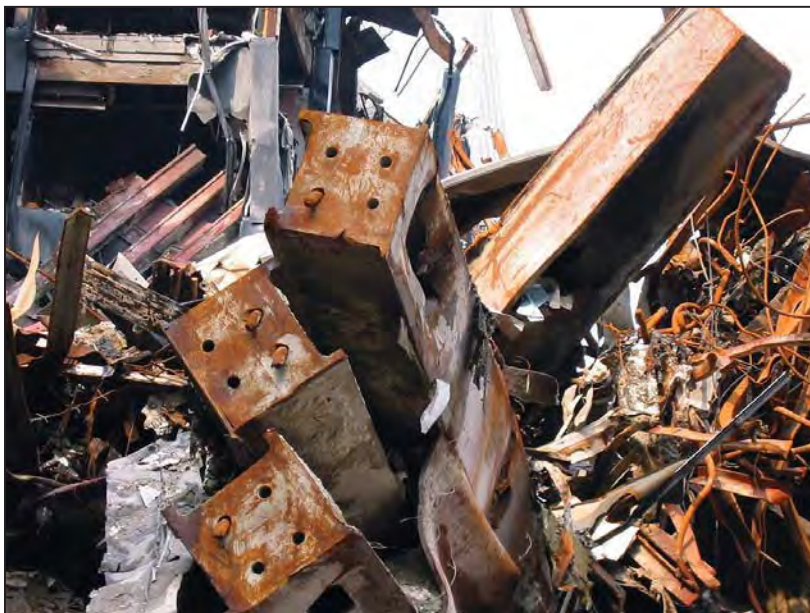
Figure B-1 Exterior column end plates.
