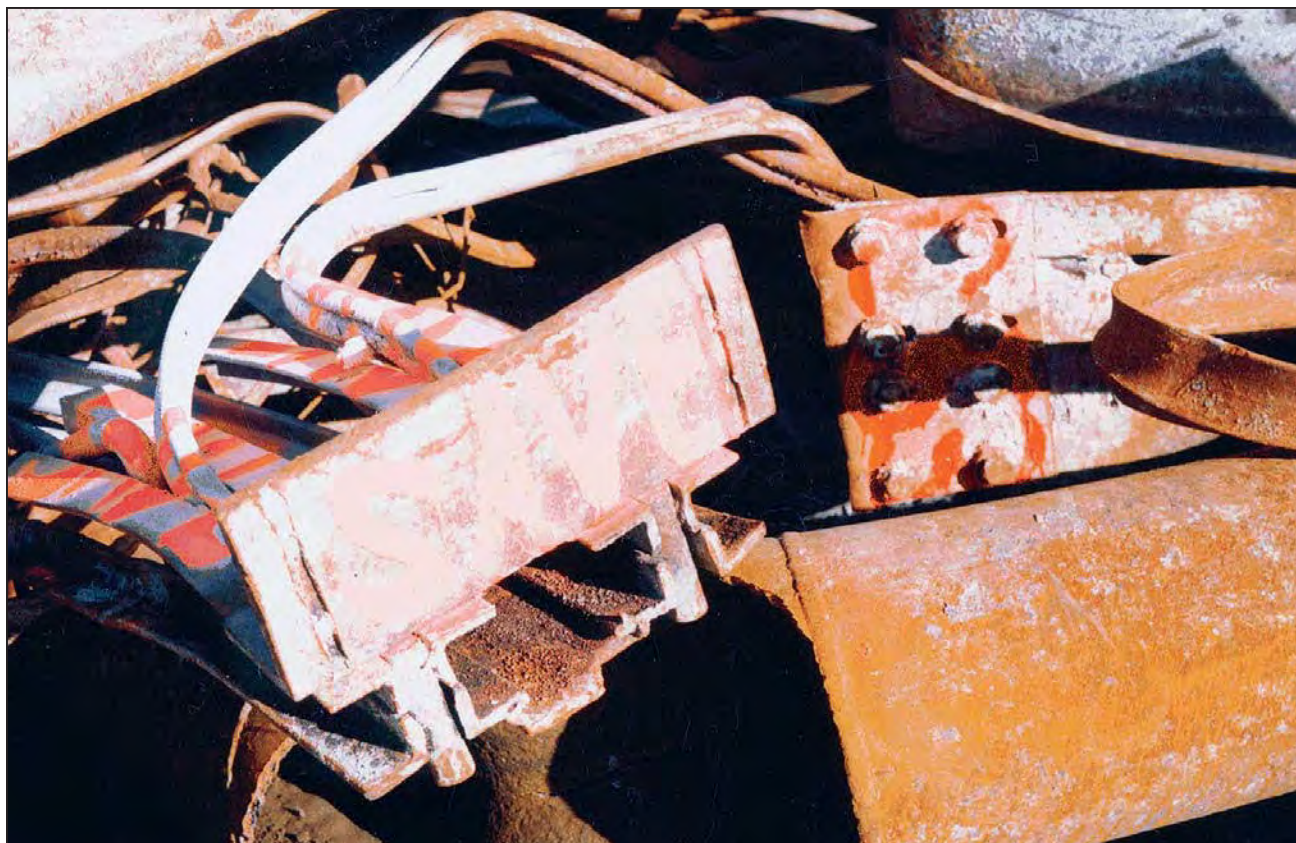
Figure D-18 WTC 1 or WTC 2 floor-truss section with seat connection fractured along welds.
