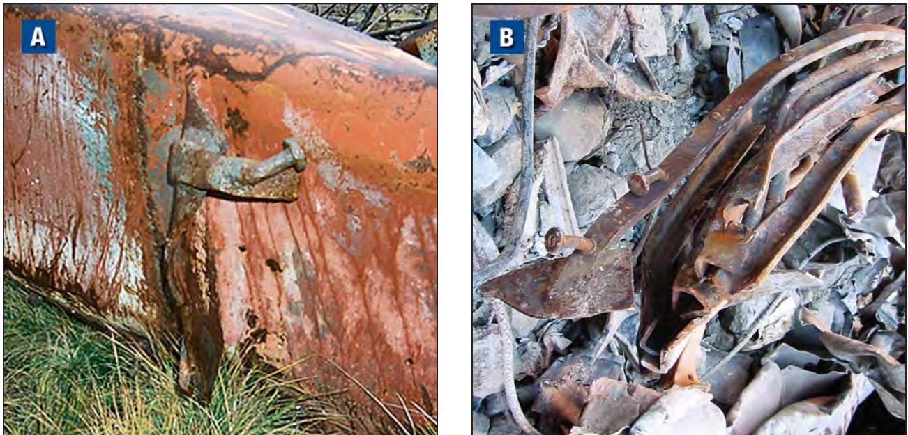
Figure B-10 (A) Bracket plate welded to the column/spandrel plate and (B) horizontal plate brace with shear connectors welded to the failed bracket.
