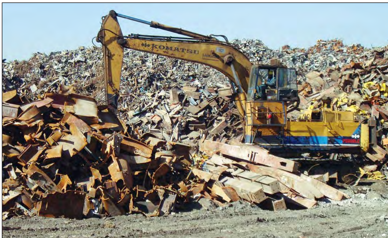
Figure D-3 Pile of unsorted, mixed steel (background) with sorted, large steel pieces (center) being lifted and cut into smaller pieces (left).
