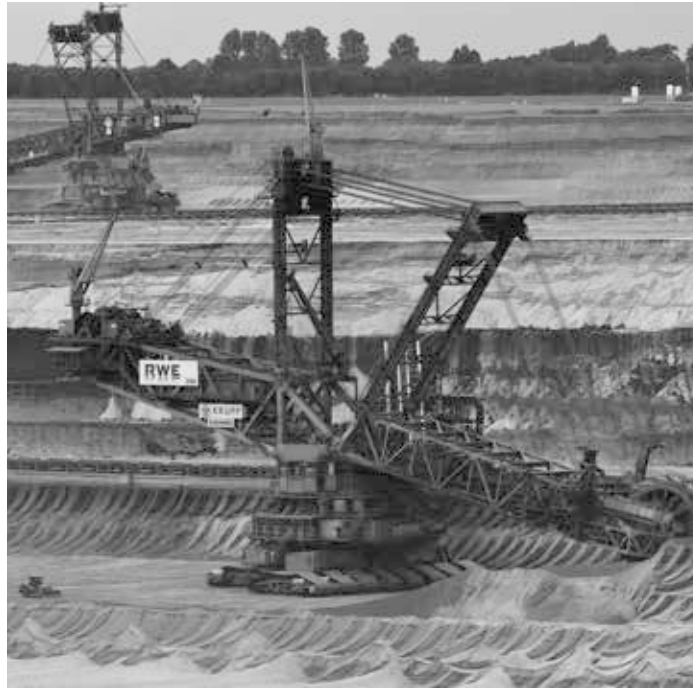
Schaufelradbagger in Garzweiler Tagebau, Deutschland. By © Raimond Spekking (via Wikimedia Commons), CC BY-SA 4.0, https://commons.wikimedia.org/w/index.php?curid=26908766
